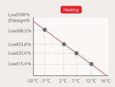
The new seasonal measurement procedure for the cooling and heating mode take the following aspects into consideration: four seasons, three EU climate zones in heating mode, partial load operation, thermostat-off consumption, stand-by consumption and crank case heater. This assesses the energy efficiency using a realistic average usage rate for a split air conditioning system.
